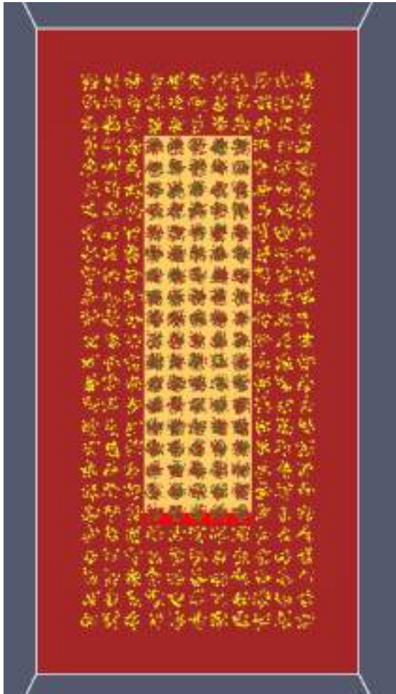
Figure 67. Trees inserted to base case domain. Trees with yellow dots are inert and only act as wind shield.
