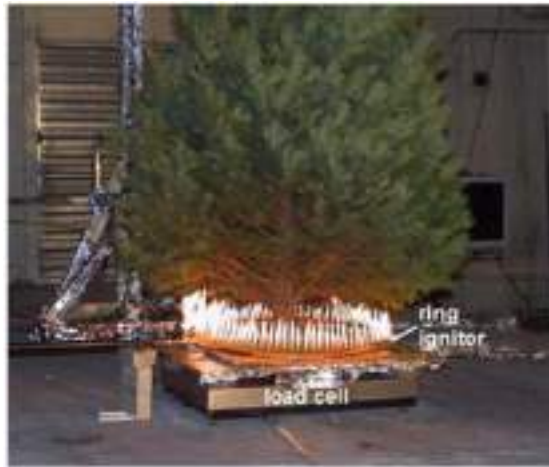
Figure 34 A snapshot from a 2 m tall tree experiment showing the igniter and load cell configuration (Mell et al. 2009).
