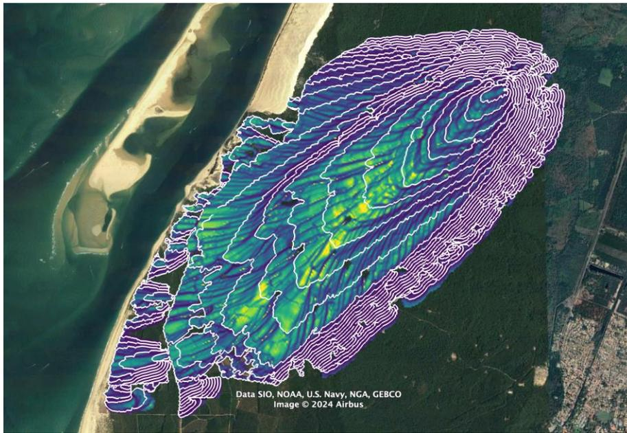
Figure 18: Fire propagation is illustrated using a color map proportional to the velocity of propagation (yellow=high, blue=low).
