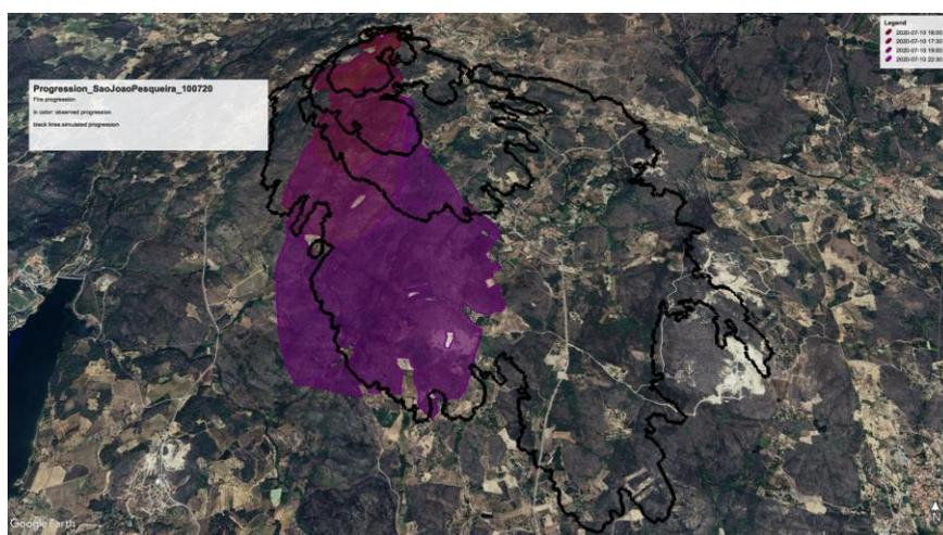
Figure 8: Observed propagation of the wildfire (in colour) with the corresponding fronts obtained in the simulation (thick black lines) The legend is in local time.
