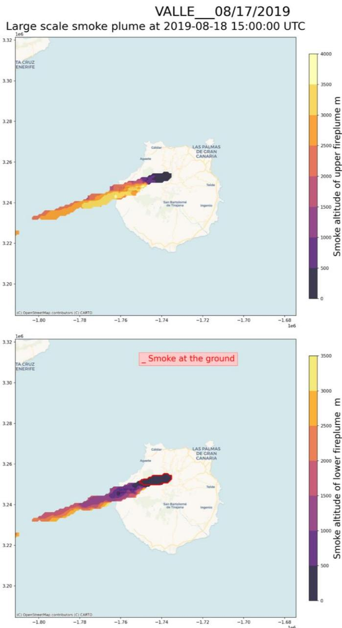
Figure 34: Type 3 plot: Smoke altitude at large length scale. Top figure illustrate the altitude of upper surface of the smoke cloud, while the bottom figure displays the altitude of the lower surface of the plume, with evidence of the smoke at the ground, which is highlighted in red.
