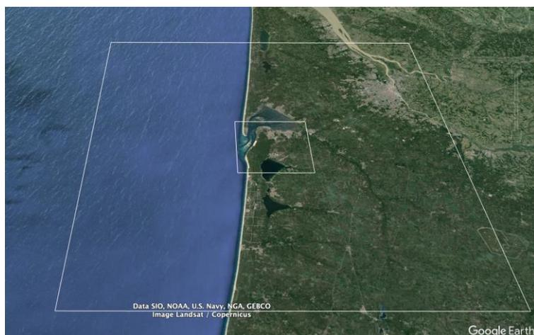
Figure 15: Domains used for the simulation. The inner domain has a higher resolution and is coupled with a fire propagation code.
