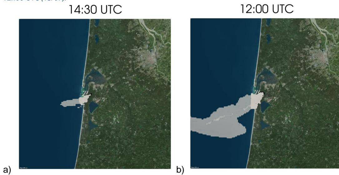
Figure 20: Fire plume 2 hours after the start of the fire (top) and at the end of the simulation (bottom).
