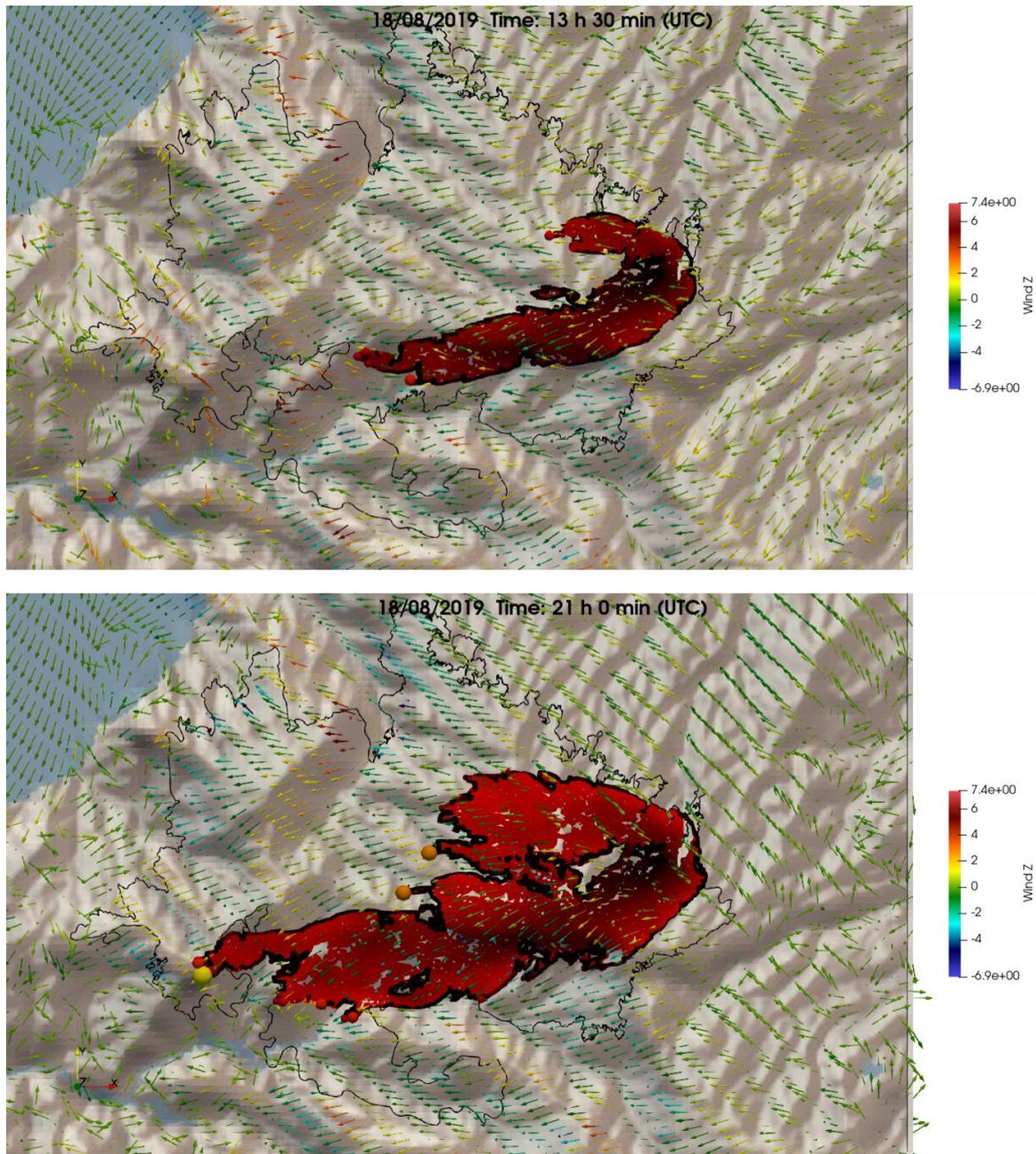
Figure 28: Surface wind field (coloured arrows) along with the propagating fire fronts (illustrated with dots whose size is proportional to the propagation speed). The simulated burned area within the fronts is color coded by time of burning. The illustrated snapshot refers to 2019-08-17 13:30:00 UTC and 2019-08-18 21:00:00 UTC. The thin black contour shows the total burned observed area for comparison.
