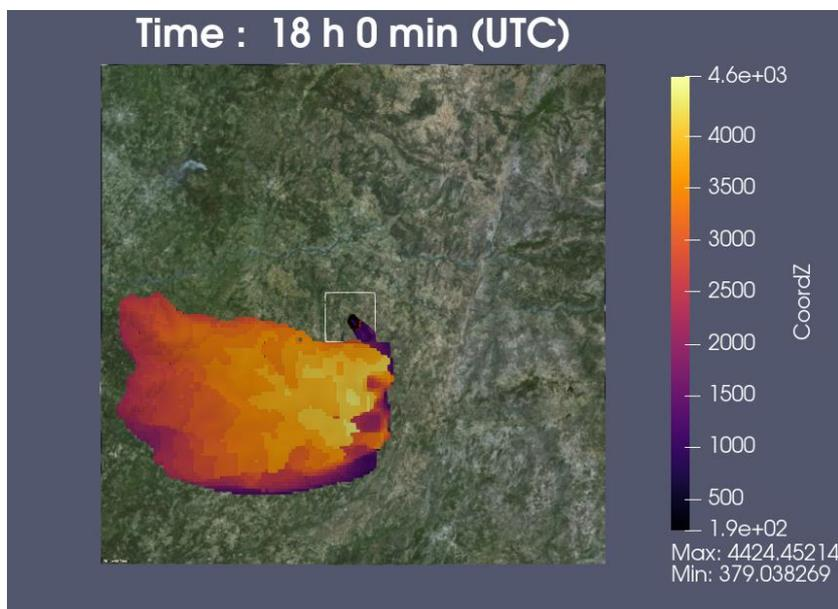
Figure 14: Global shape of the fireplume at 18:00 UTC. The colour scale indicates the plume elevation.
