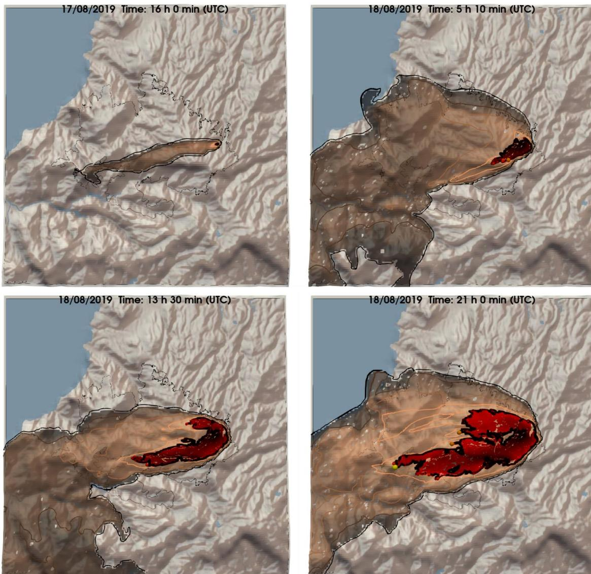
Figure 29: Surface smoke concentration (orange to brown concentration) along with the propagating fire fronts (illustrated with dots whose size is proportional to the propagation speed). The simulated burned area within the fronts is colour coded by time of burning. The illustrated snapshot refers to 2019-08-17 13:30:00 UTC and 2019-08-18 21:00:00 UTC. The thin black contour shows the total burned observed area for comparison.
