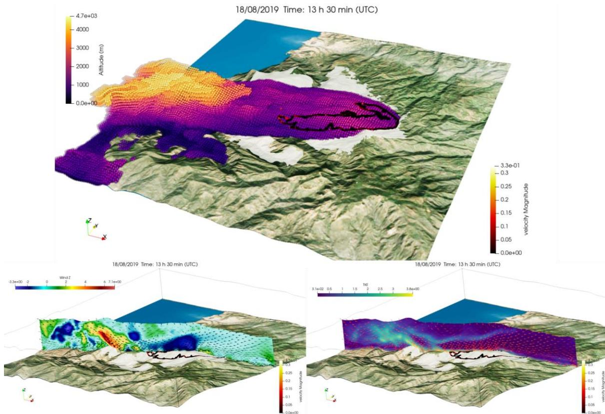
Figure 30: 3D view of the smoke plume at 2019-08-17 13:30:00 UTC, the color coding is proportional to the plume altitude. In the lower part of the figure two sections along the plume axis show the vertical wind field (left) and the turbulent kinetic energy (right). The fire fronts are also highlighted.
