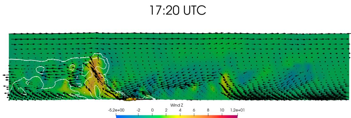
Figure 22: Vertical section showing the contours of the fire plume (in white) and the wind field. The colour scale indicates the vertical component of wind speed..
