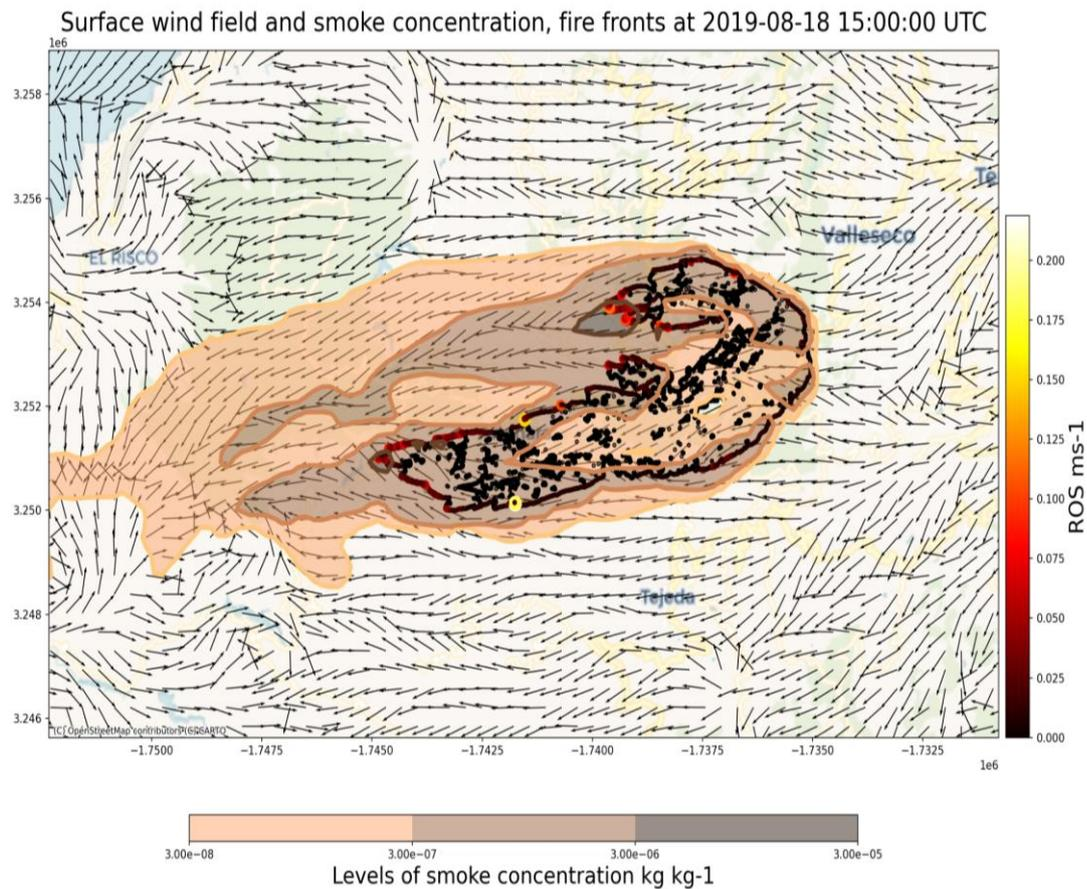
Figure 33: Type 2 plot: Smoke concentration at the ground (kg/kg-1) is illustrated using orange contours. The direction of the surface wind field is illustrated with black arrows. The fire front is illustrated using point sizes proportional to the ROS (ms-1).
