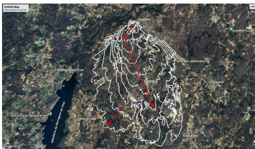
Figure 9: Simulated wildfire front (thick white contours). The time between the displayed contours is 1 h. The arrows highlight the main changes in the propagation direction.
