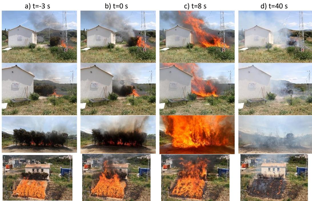
Figure 14: Photographs of the burning phases of rockrose hedge a) Fire spread in wood wool; b) Hedge ignition. c) Hedge burning and d) Hedge extinction.
