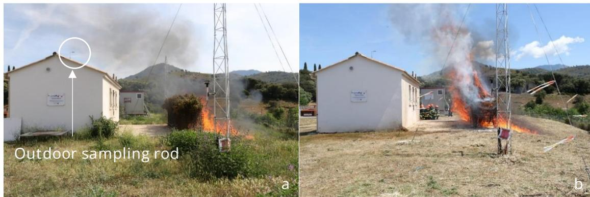
Figure 21: Photographs of the hedge burning of a) rockrose b) cypress equipped with smoke analysers
