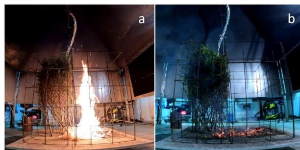
Figure 28: Different phases of an experiment with a fuel MC of 100 % - a) Fire front across the wood wool bed b) No ignition of the branches
