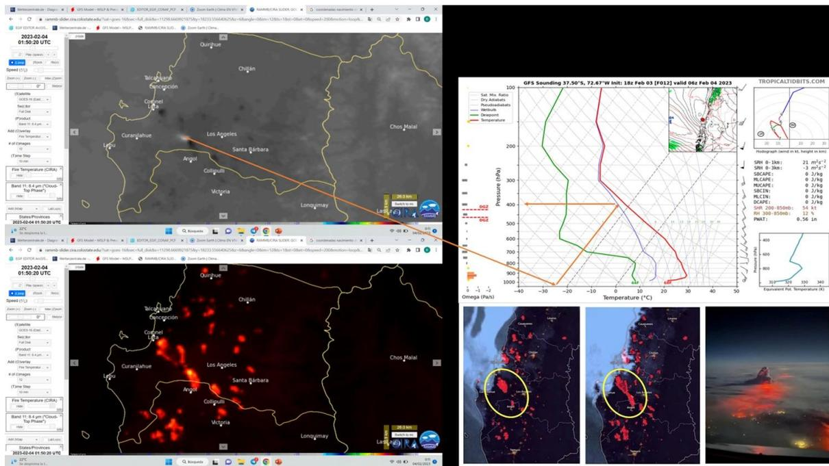
Annex Figure 7. Determination of the height convection column using the GOES 16 satellite and radiosondes of GFS model.
