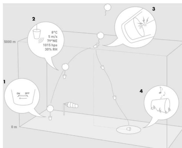
Fig. 2. Overview of how Windsond works
