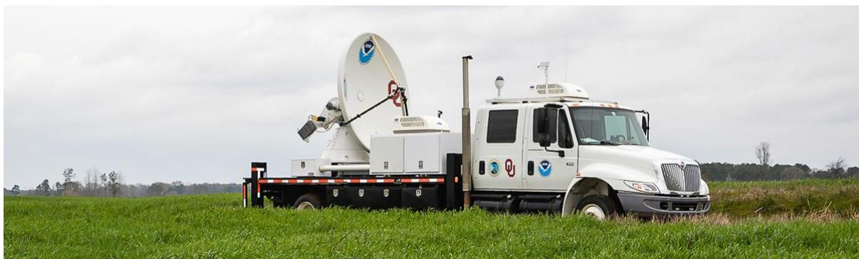
*Image 3. Example of mobile radar. NOAA X-POL radar used to study tornadoes, hurricanes, dust storms, winter storms, mountain rainfall, and even swarms of bats (Source: <https://www.nssl.noaa.gov/tools/radar/mobile/>)*
