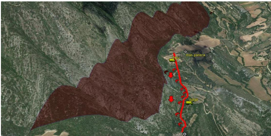
Figure 8. Proposal Sketch for an implementation of the use of technical fire to ensure the confinement of the fire line within the limits of the scenario resolution. On the established contention line formed by road, fields, and trails fire is used to improve the effectiveness in the weakest points. Source: Manoeuvre diagram used in 2022 Baldomar fire, Bombers (CFRS) internal use (unpublished).
