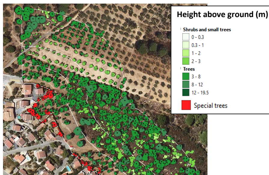
Figure 17: Individual tree detection based on local maxima region growing from a CHM, and their estimated height. Special trees (in red) are those trees whose crown is located less than 2m from a built-up plot.
